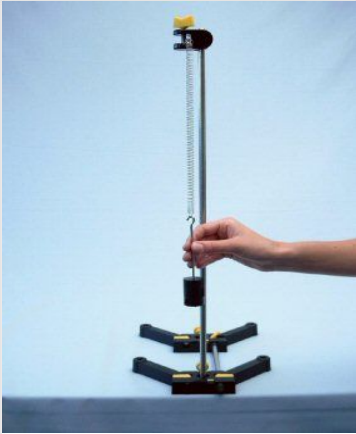
Deflecting the spring with the spring constant 20 \text{ N/m}
