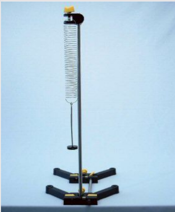
Test setup of the coil spring pendulum
