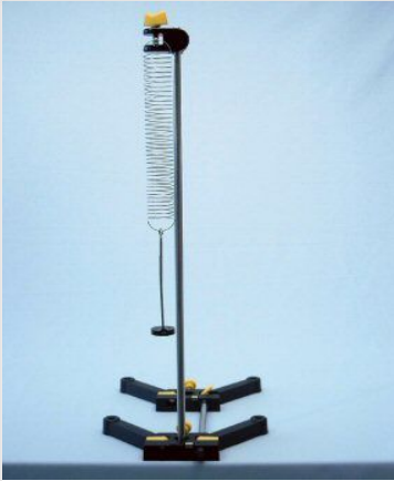
Test setup of the coil spring pendulum
