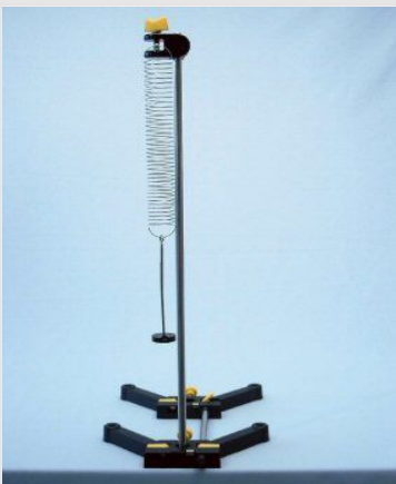
Test setup of the coil spring pendulum
